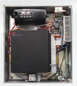
The Federal Signal UltraVoice® Remote Interface (UVRI) unit is a remote terminal unit (RTU), specifically designed to provide remote control and status monitoring of an individual buildings fire alarm panel, mass notification panel, or public address system. The UVRI establishes a communication link between an isolated building unit and its mass notification system into our Federal Commander Digital Control System, creating a fully integrated indoor and outdoor Mass Notification System.
