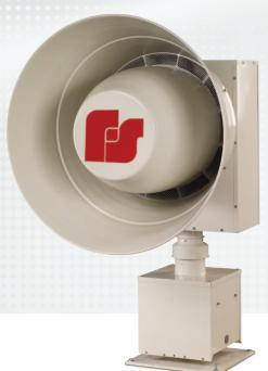
The Federal Signal 2001-130 public siren is a high power, rotating, uni-directional outdoor warning siren that offers an anechoic certified signal strength of 130 dB(C) +/- 1 dB(C) at 100-ft. The high-decibel output provides maximum coverage with minimum installation cost. Radio activation can further minimize installation costs by eliminating the need for leased dedicated control lines.
